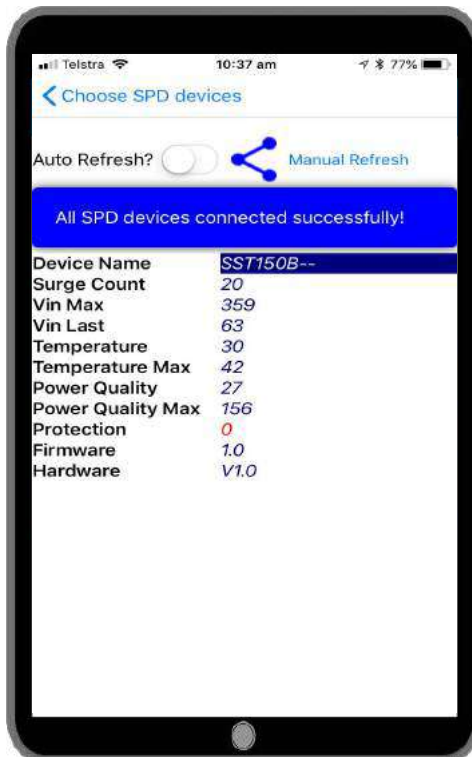
Replace as no protection is left
