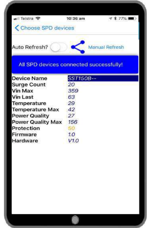
Replace as protection is reduced
